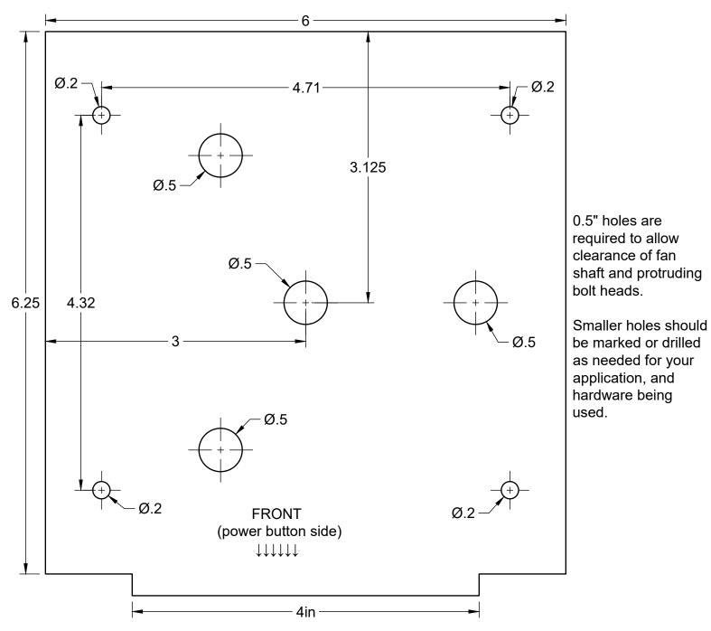
VERIFY PRINT SCALE HERE ONLY. It is exactly 4". other dimensions are approximate, and just for general reference due to a combination of Metric and SAE parts.
